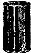
Faraday ice pail, used in demonstrating electrostatic principles.
